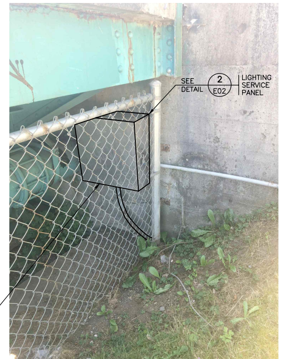
DETAIL E02 LIGHTING SERVICE PANEL N.T.S.
